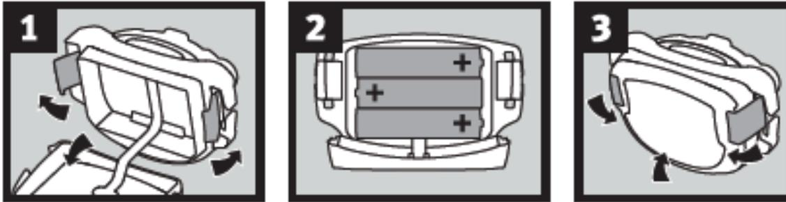
1. Release latches and open cover of battery compartment.
